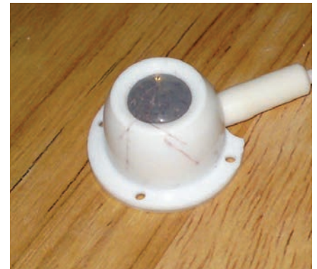
Figure 1: Misaligned needle insertion resulting in a) Port failure split in the casing and b) Needle insertion scratches against the port casing.
